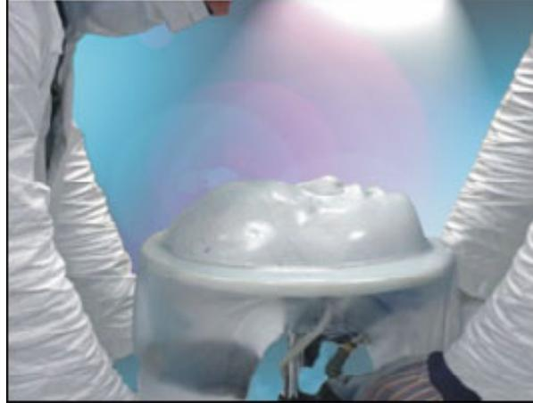
\* During any heating procedure, keep an active eye on the material as it is heating so that you can get a fully heated surface area for the pull. Many ovens will only heat the center and less on the periphery, so you need to watch the material to prevent over heating and bubbling. Sufficiently heated material should have soft, taffy like drape when picked up by hand.
